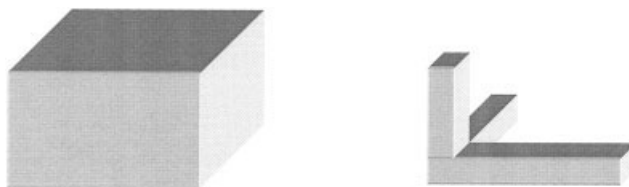
Figure 4. Parent particle and child particle with the same length, width, and depth but different shape factors.
